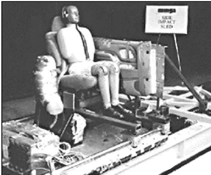
The calm before the storm: BioSID crash impact dummy awaits side impact outfitted with six SpaceAge Control Model 160-0321L position transducers.
