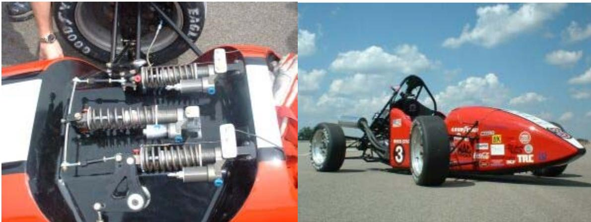
Left: Series 150 displacement units measure shock travel.
