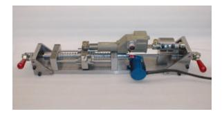
SpaceAge Control D60 digital output dispacement sensor monitors actuator final assembly fixture.
