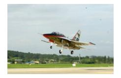
KAI's T-50 next generation jet trainer lifts off for the first time with the nose-mounted 4-vane 100700-03 air data boom.
