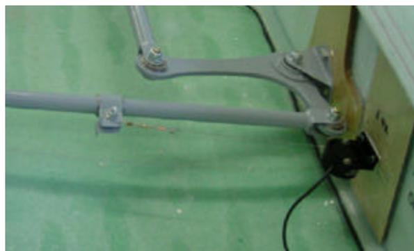
Series 173 position transducer installed to measure aileron movement.
