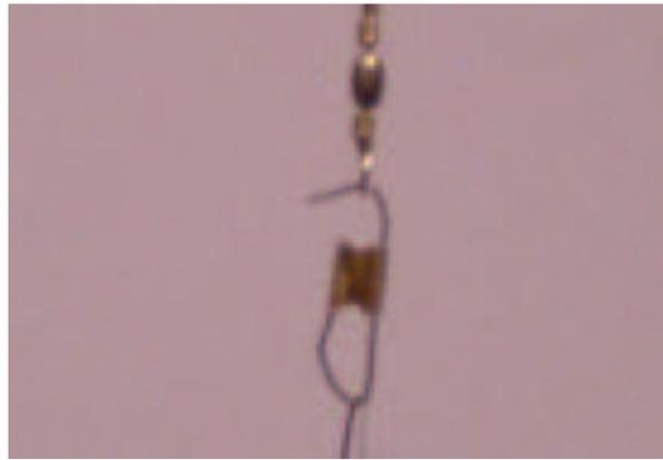
Typical swivel failure mode
