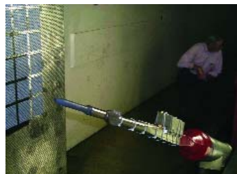
300643 heated probe undergoing low- and high-speed wind tunnel testing
