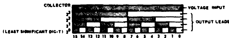
Fig. 6.0-2 Principle of a rectilinear type shaft position encoder
